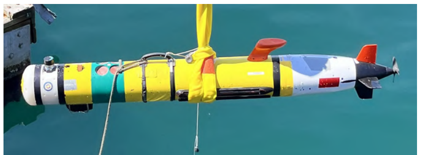
ISS360 Sonar (far left) Installed on the REMUS-100 AUV
