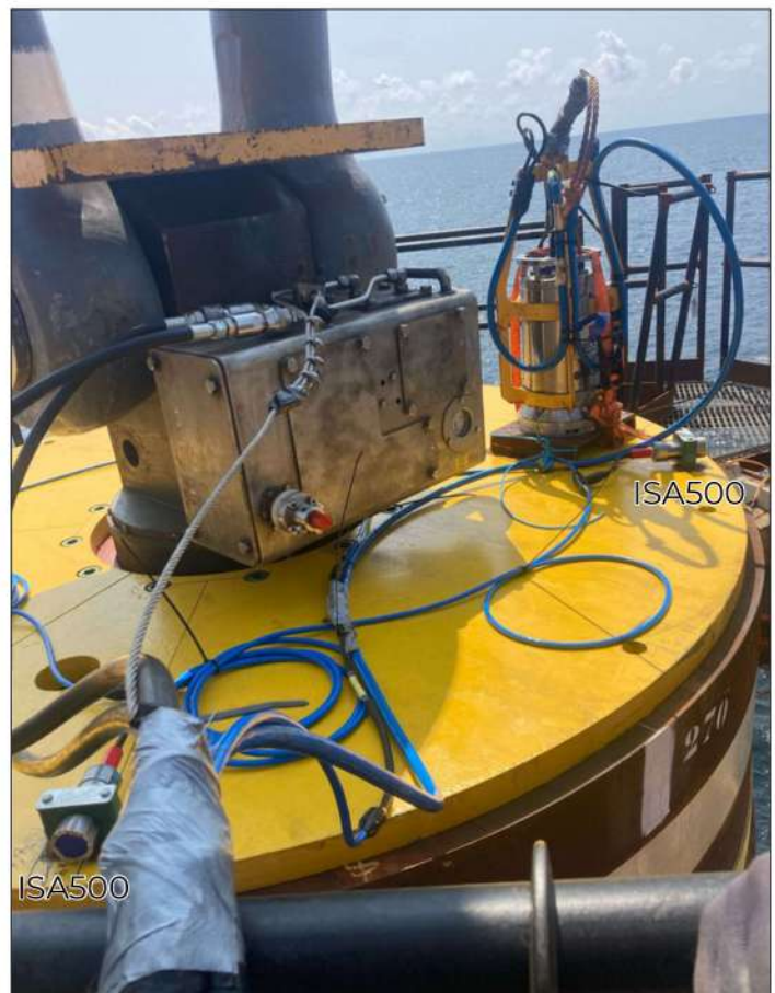
ISA500 mounted around the top of pile. Source: JK -Hydroconsult
