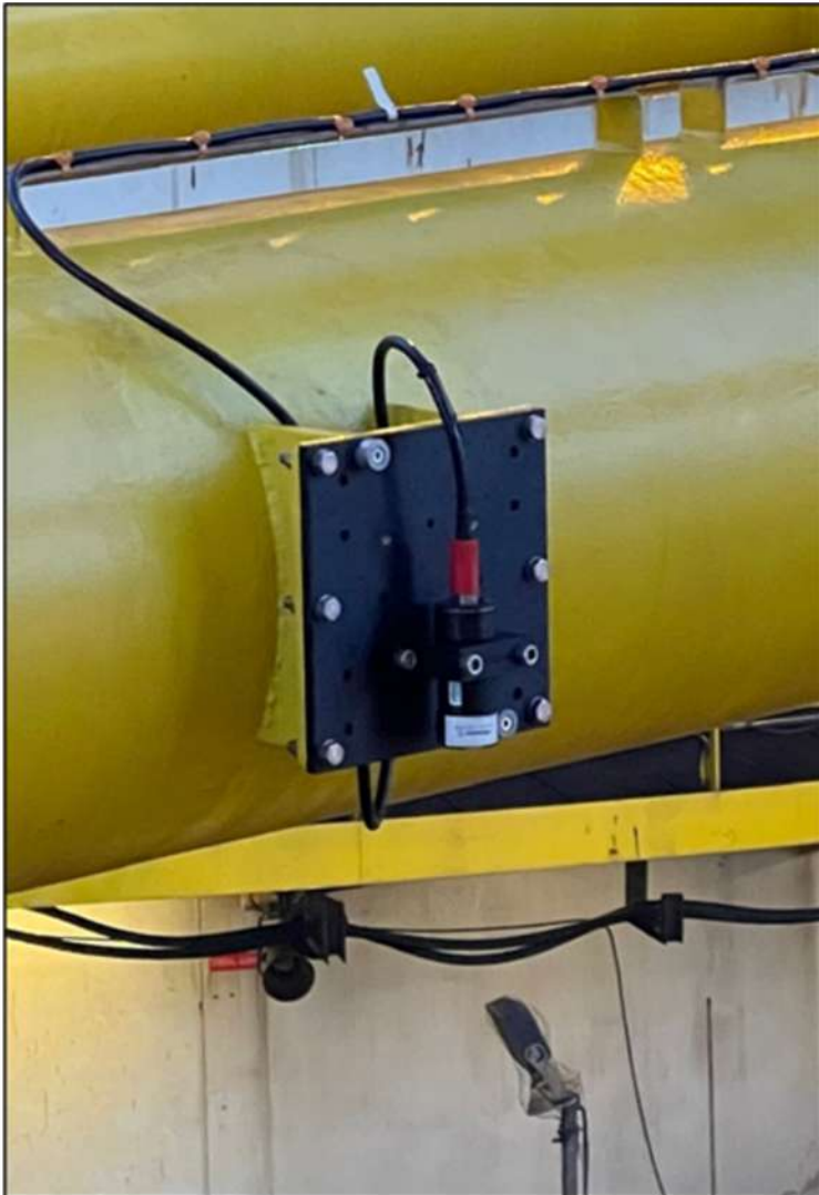
ISA500 Altimeter mounted onto Subsea Template
