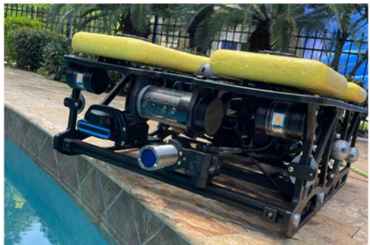
ISFMD sensor installed on the ROV-3000.
