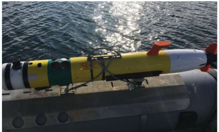
ISS360 Sonar (far left) Installed on the REMUS 100 AUV
